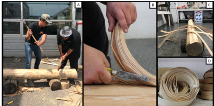
Figure 1: The process of preparing black ash splints for W8banaki basketry. Photo by Laurence Boudreault
